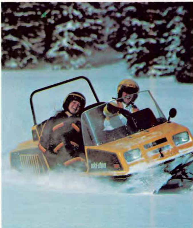
Two can ride as easily as one in this new side-by-side bucket seat Elite snowmobile by Ski-Doo, the industry's first built-to-order machine. It features rear liquid-cooled engine, full instrumentation, forward-reverse gear, comes made to order with buyer's monograms.
